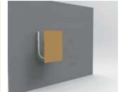
9. Removal of the cardboard support.
