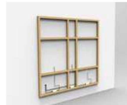
1. Create the supporting frame and provide for power connections for the individual letters.
